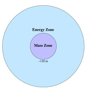
Figure 1: The two zones of a Cherenkov lateral distribution from an EAS, as seen from along the shower core. The inner ("mass") zone is sensitive to primary mass and energy, while the outer ("energy") zone is sensitive mostly to primary energy. The outer radius of the energy zone is determined by the energy of the shower and the threshold of the detector.
