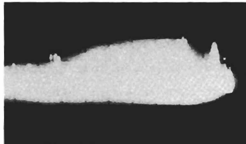
Fig.14 Display of spectrum analyser, illustrating the momentum spread of captured beam by the frequency sweep of 380 \text{kHz} .
