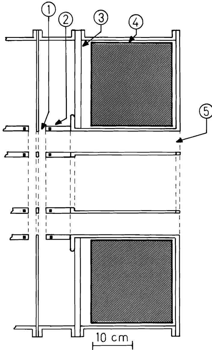
Figure 1. Pulselac C Acceleration Module. 1) Magnetically insulated acceleration gap. 2) Coaxial drift tube structure with magnetic coils. 3) Vacuum insulator. 4) Ferrite core (250 kV, 50 nsec). 5) Annular drift region.
