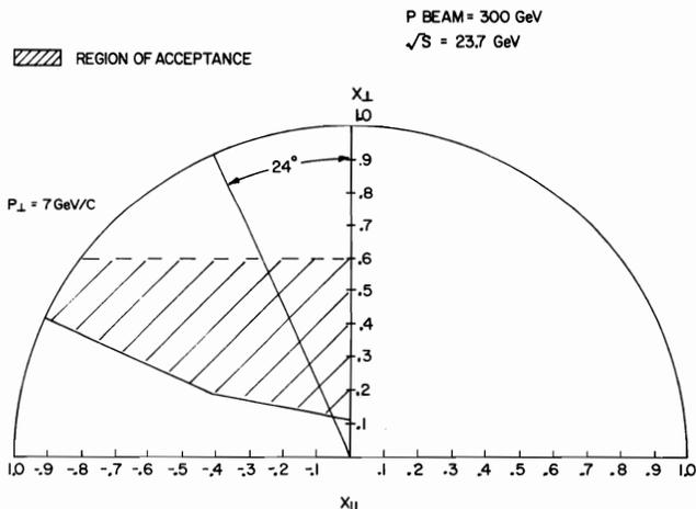
Fig. 4 Shaded region is the region of acceptance at 300 GeV. The acceptance of the spectrometer at a single forward angle setting of the spectrometer ( $\sim 6^\circ$  in the laboratory) is indicated by the  $24^\circ$  cms slice.
