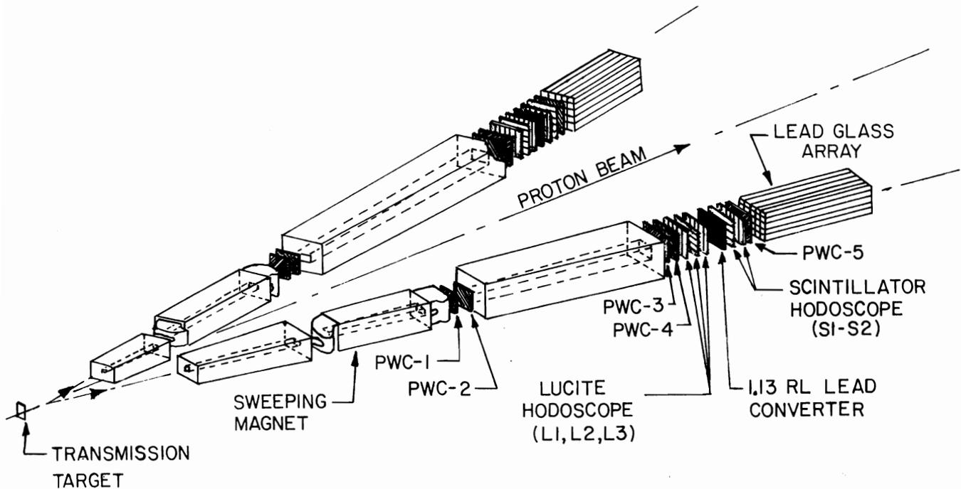
Fig. 3 Schematic view of the double arm photon spectrometer.
