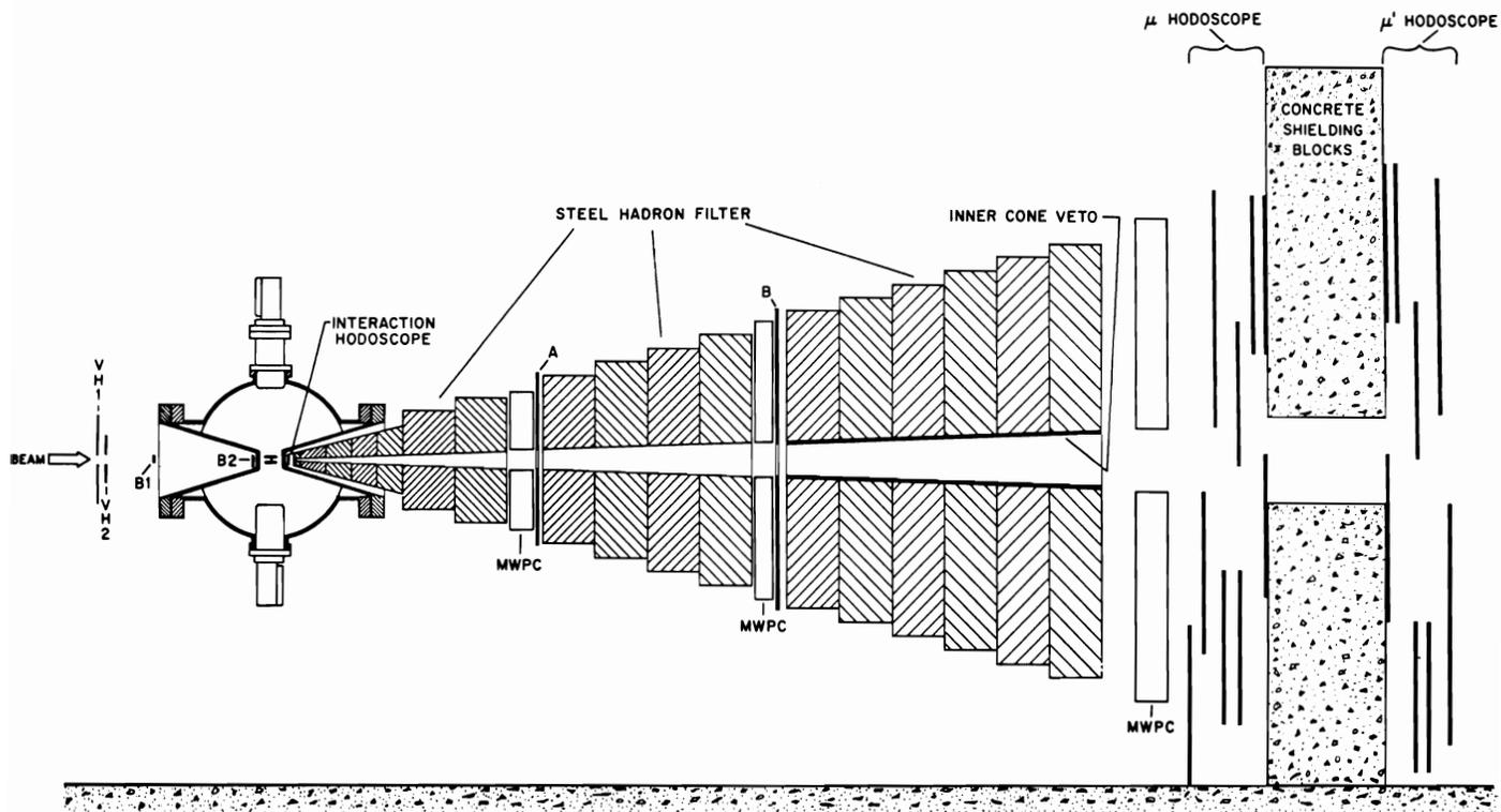
Figure 7. Arrangement of Yale - Fermilab experiment.
