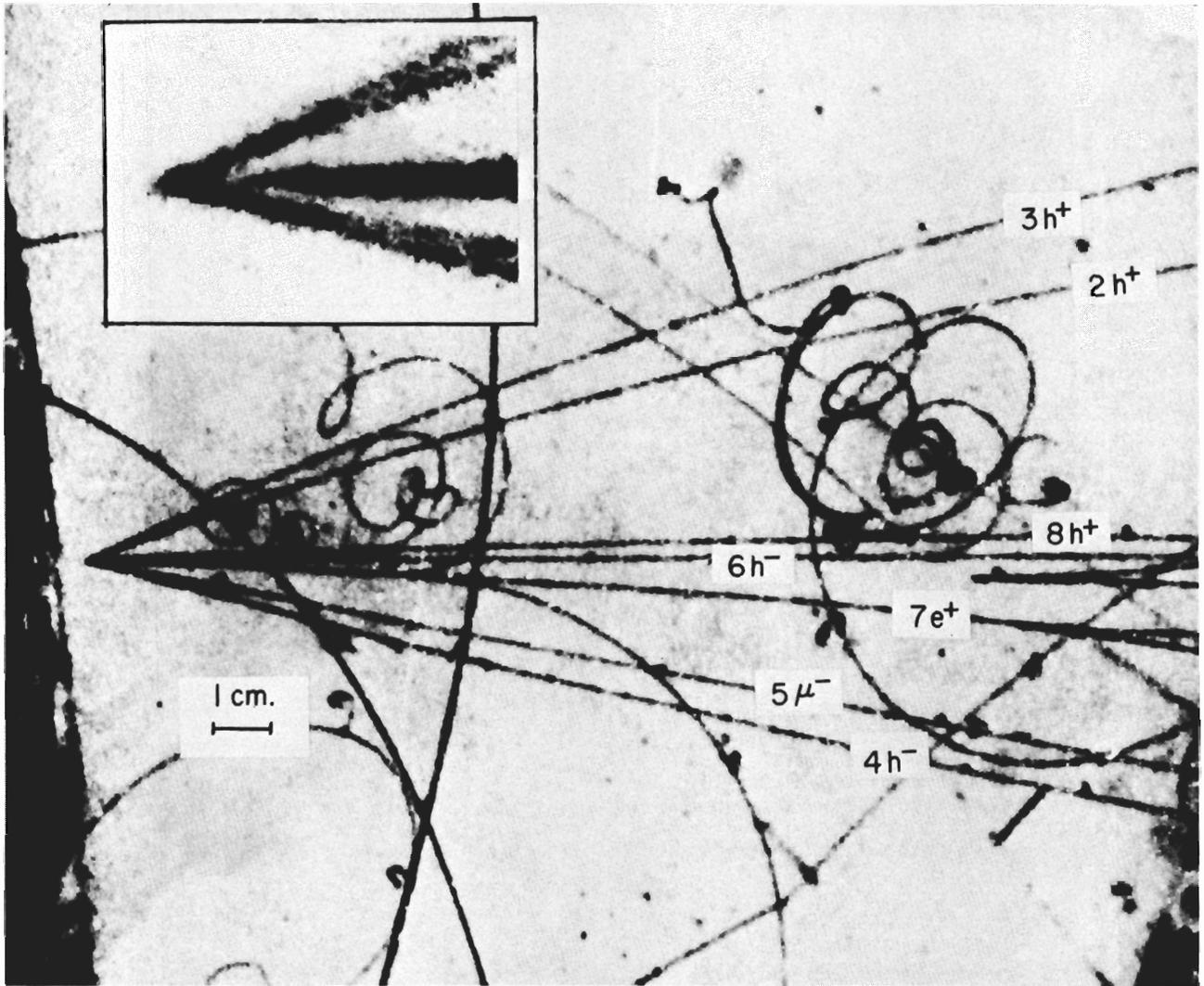
Figure 2. Candidate event for charm decay obtained in 15' Bubble Chamber (BFHSW)
