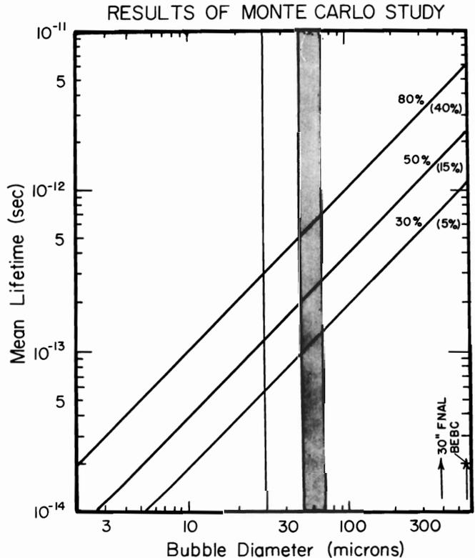
Figure 13. The relation between lifetime sensitivity and bubble diameter in LEBC.
