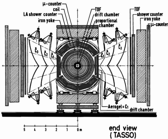
Fig.1 The TASSO detector viewed along the beam.
