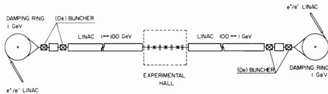
Fig. 4 The superconducting linacs of Gerke and Steffen use two superimposed damping rings at each end to cool the slowed-down electron and the positron bunches before re-use (Ref. 21).
