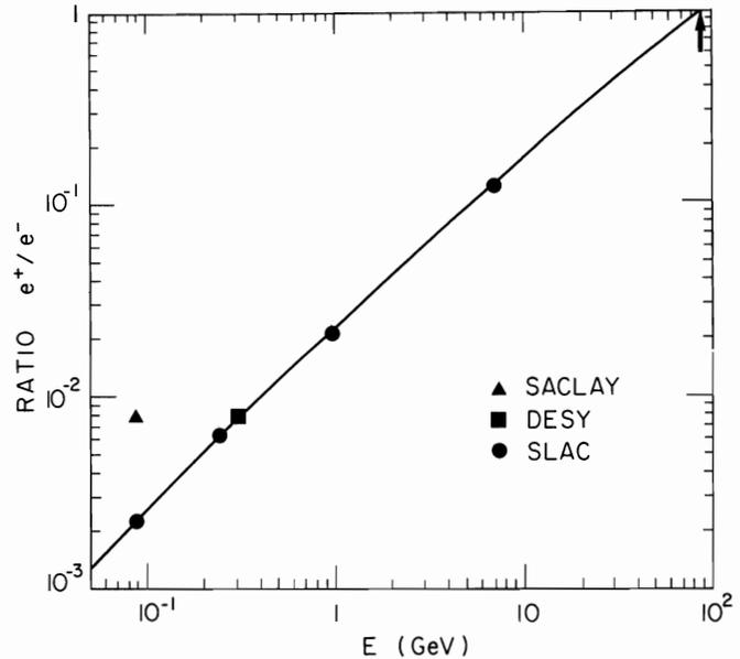
Fig. 10 Yield of positrons as a function of the energy of the electrons impinging on a target of 1-2 radiation lengths (the optimum thickness varies logarithmically with energy). The points from Saclay<sup>38</sup> and DESY<sup>39</sup> are measured with collectors of different acceptances. The points of SLAC have been computed with a very sophisticated program and the line extrapolates them to higher energies.
