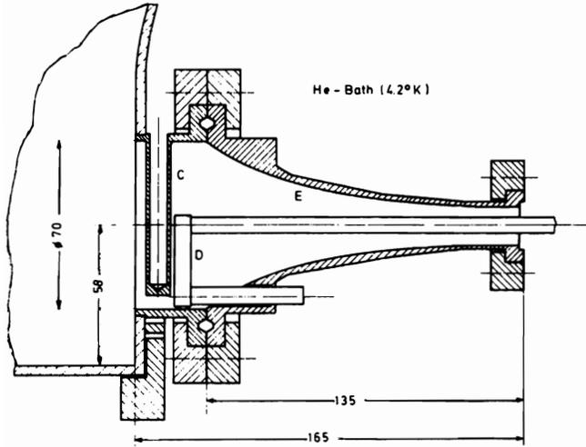
Fig. 6 Higher-mode coupler designed by the Karlsruhe group for the superconducting cavity to be installed in DESY.
