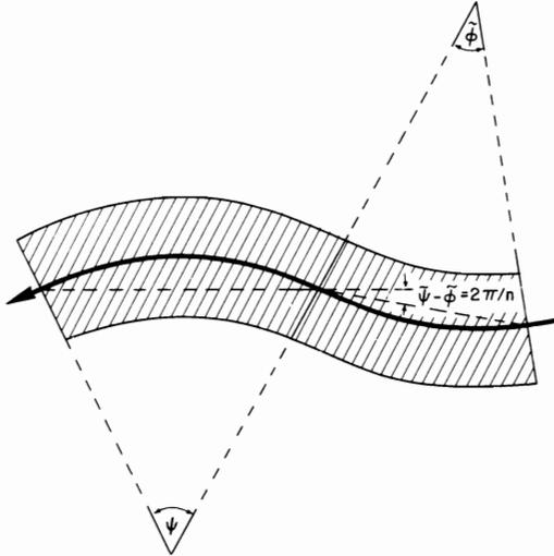
Fig. 3 One cell of the 1 GeV Wiggler storage ring proposed by Steffen to cool electron and positron bunches (Ref. 27). The angles are  $\phi = 0.25$  and  $\psi = 0.27$ , and the number of 1 m long cells is 300.
