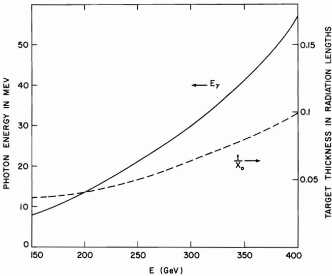
Fig. 9 Energy dependence of the photon energy produced in a wiggler of 2.5 cm wavelength and 0.37 T field. The dashed curve gives the target thickness needed for a 100 m wiggler to produce one low-energy positron per electron.
