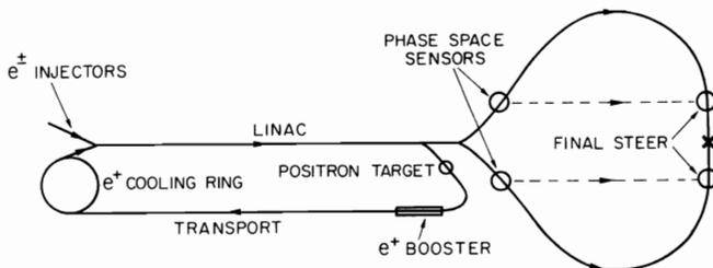
Fig. 14 Scheme of the Single Linac Collider proposed by Richter
