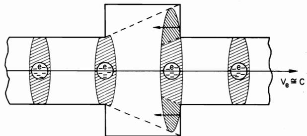
Fig. 5 Schematic representation of the physics behind the phenomenon of the higher-order mode losses.
