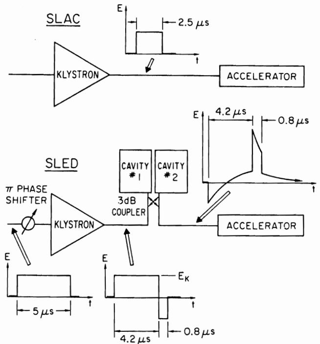
Fig. 15 In the SLED scheme the RF pulse is shortened and the peak field increased by adding a 180° phase shifter and two cavities with a 3 dB coupler.
