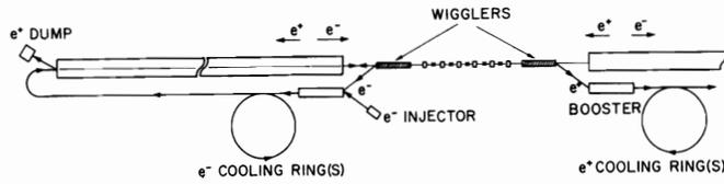
Fig. 8 In this scheme<sup>37</sup> the energy is recovered but the particles are not. The low-energy positrons and electrons are produced by the photons radiated by the beams in wiggler magnets.
