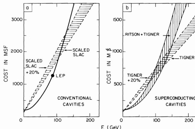
Fig. 12 The costs of conventional and superconducting colliding linacs are compared with the cost of optimized storage rings. The many assumptions that go into this comparison are listed in the text.
