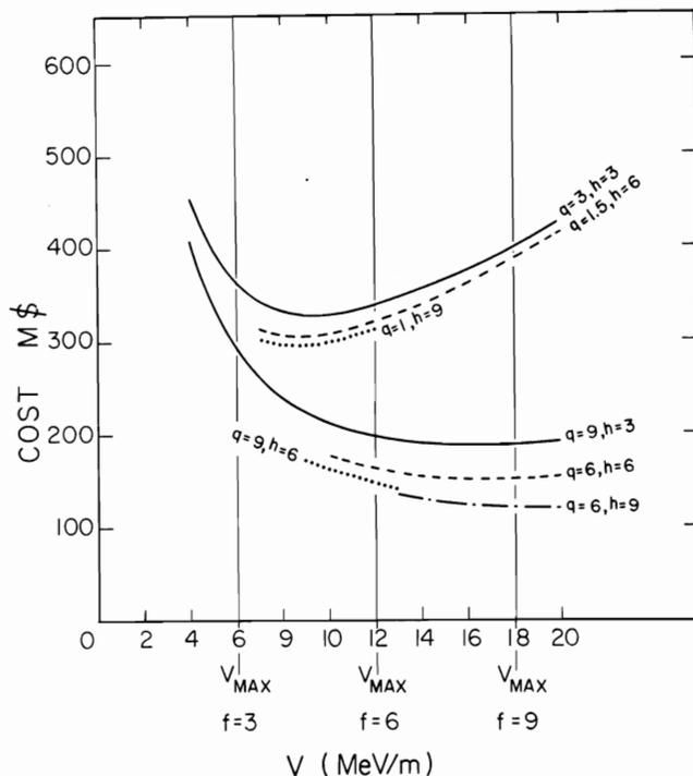
Fig. 13 Cost of superconducting linacs versus the voltage per unit length as estimated by Tigner<sup>28</sup>. In this figure  $q$  is the Q-value measured in units of  $10^9$  and  $h$  the RF frequency  $\nu$  measured in  $10^9$  Hz. Present technology has  $qh \approx 9$ . The cost is given for a 100 GeV linac.
