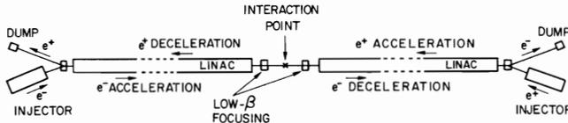
Fig. 2 Working principle of colliding linacs with recovery of the beam energy. For simplicity, in this drawing it is supposed that electron and positron bunches can be directly produced from an injector with small emittances.
