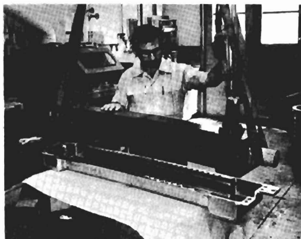
Fig. 6. Support Structure and Coils After First Potting.
