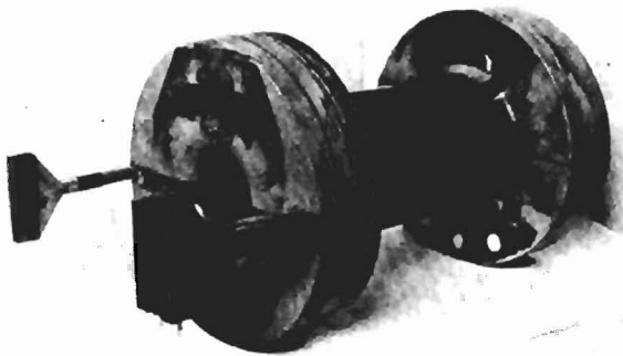
Fig. 8 Impregnated coil system of Rutherford Laboratory pulsed dipole model AC3
