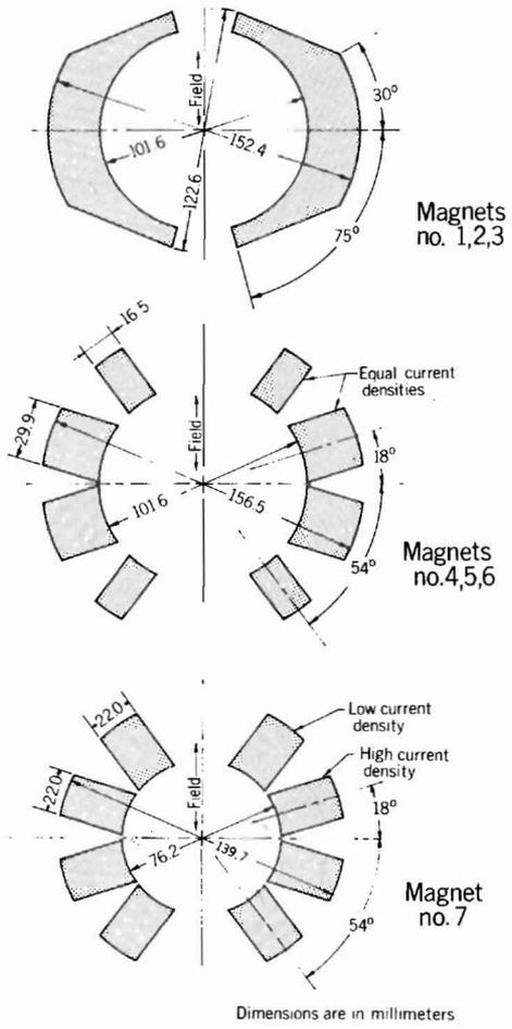
Fig. 3. Winding cross-sections.
