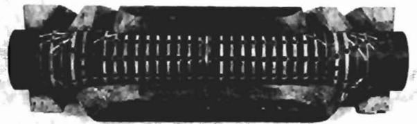
Fig. 6. Winding form for Magnet #7.
