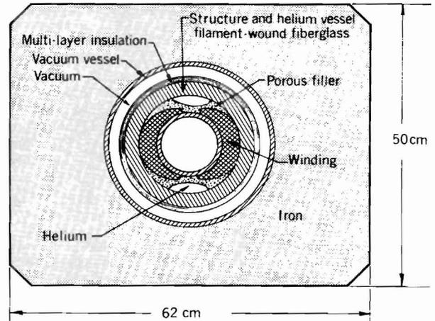
Fig. 1. Reference design for a superconducting synchrotron magnet.
