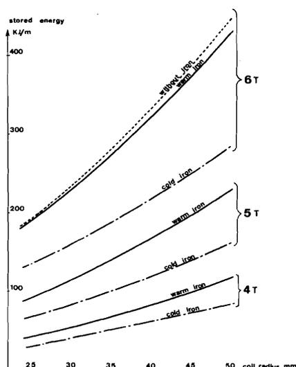
FIG.4- Stored energy as a function of the aperture.
