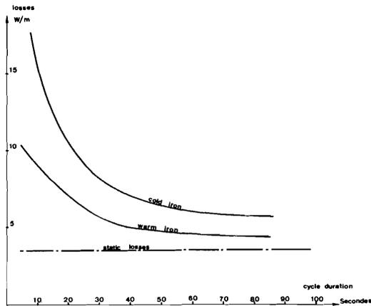
FIG.5- Helium temperature losses as a function of the cycle duration.
