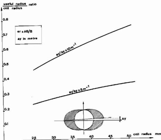
FIG.2- "Bad field" margin coming from the quadrupolar error.
