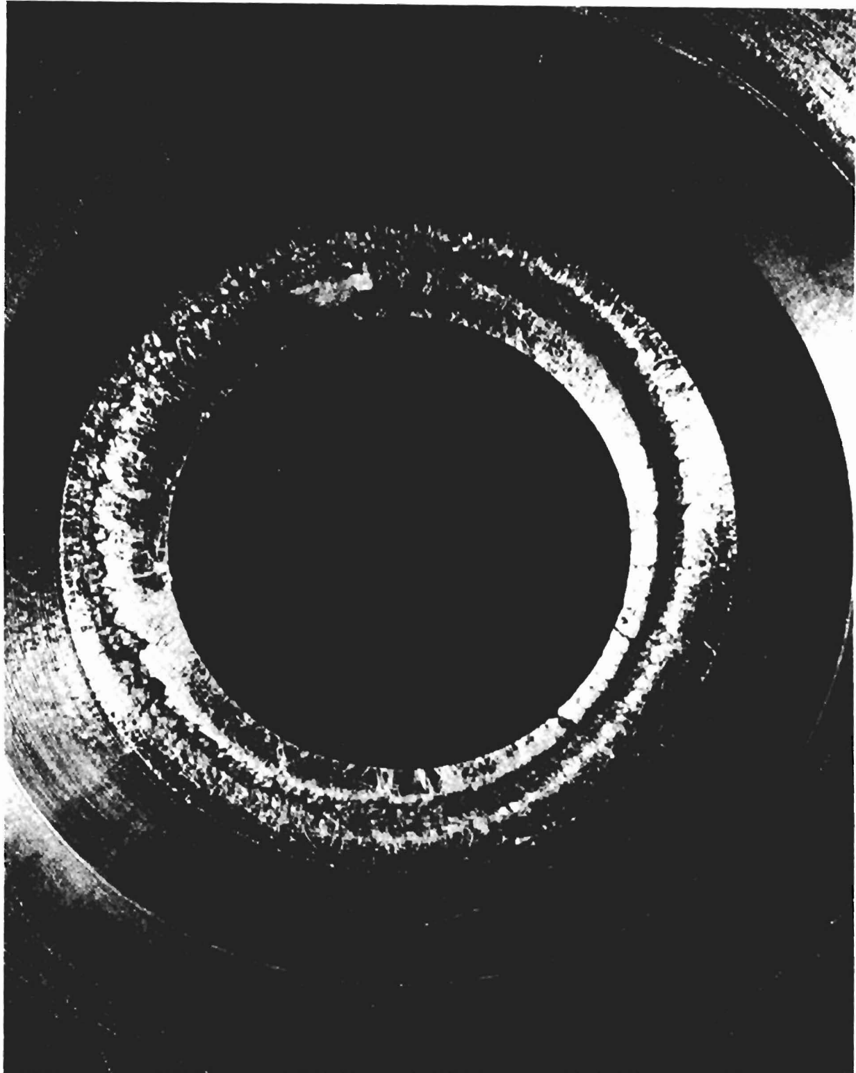
Figure 12. Beam damage on 2-inch positron target.
