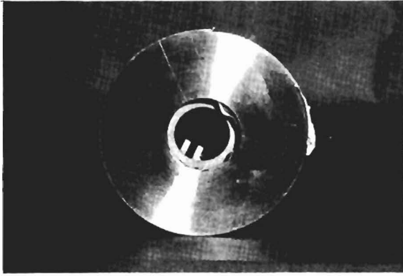
Fig.2a Tape coil fabrication.
