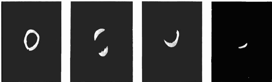
Figure 3 (b) - Tungsten screen photographs showing beam rotation and rf chopping at S-band frequency.
