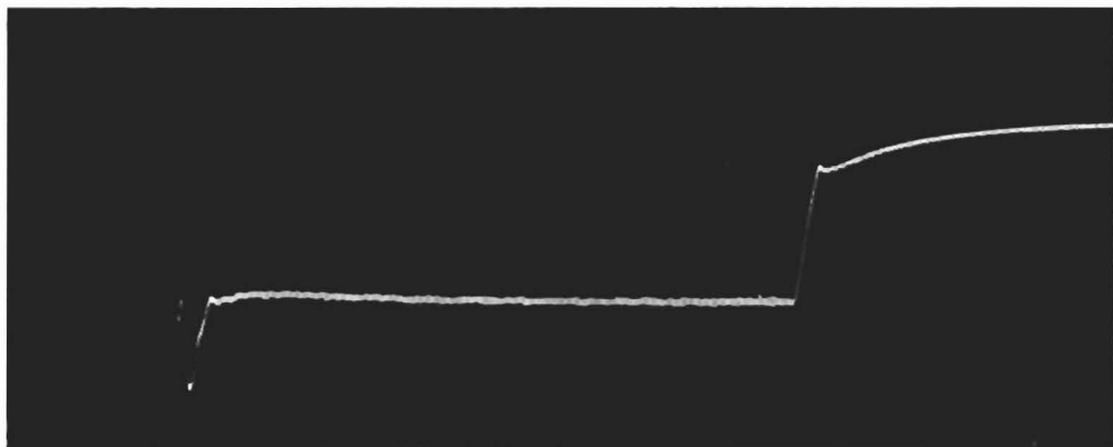
Fig. 7. Arc current, about 12 A after initial peak of 500 \mu sec pulse.
