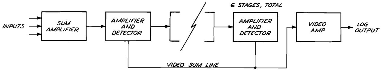
Figure 9. Logarithmic if Amplifier of Progressive Detection Type
