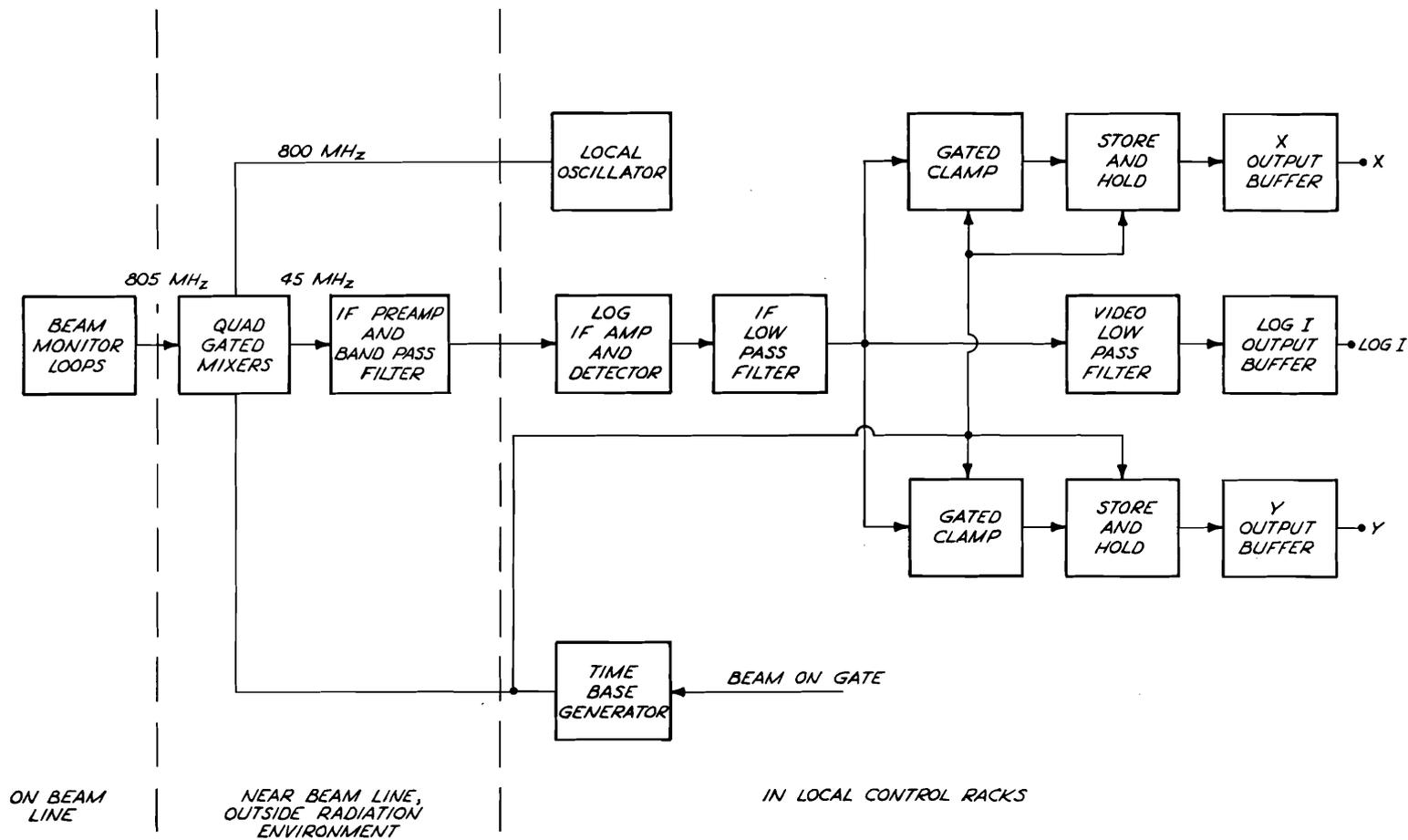
Figure 5. A Practical Beam Position Monitor System
