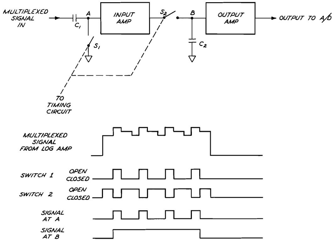
Figure 10. Simplified Diagram of the De-multiplexing Circuit
