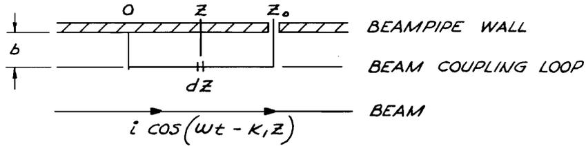
Figure 3. Emf Induced by Beam in a Loop
