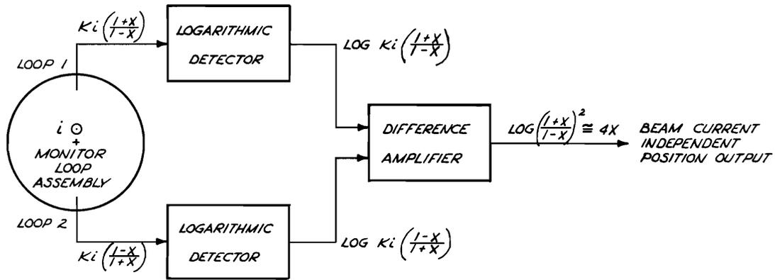
Figure 2. Basic Principle of Beam Position Monitor System
