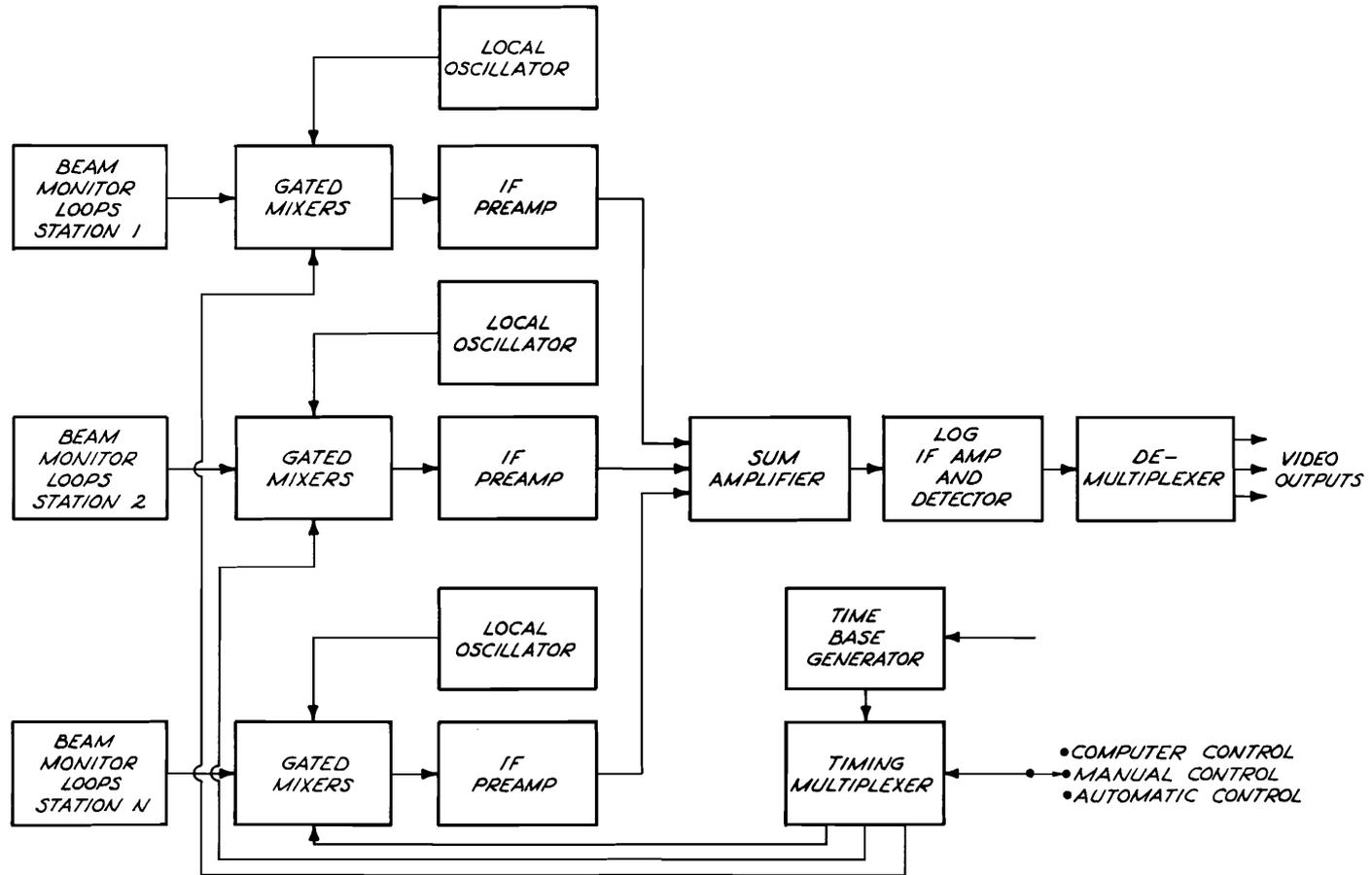
Figure 6. Practical System with Multiplexing Added
