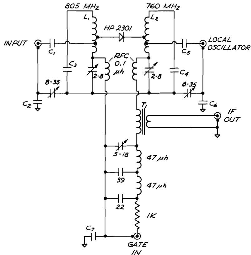
Figure 7. Schematic of 805 MHz Gated Mixer
