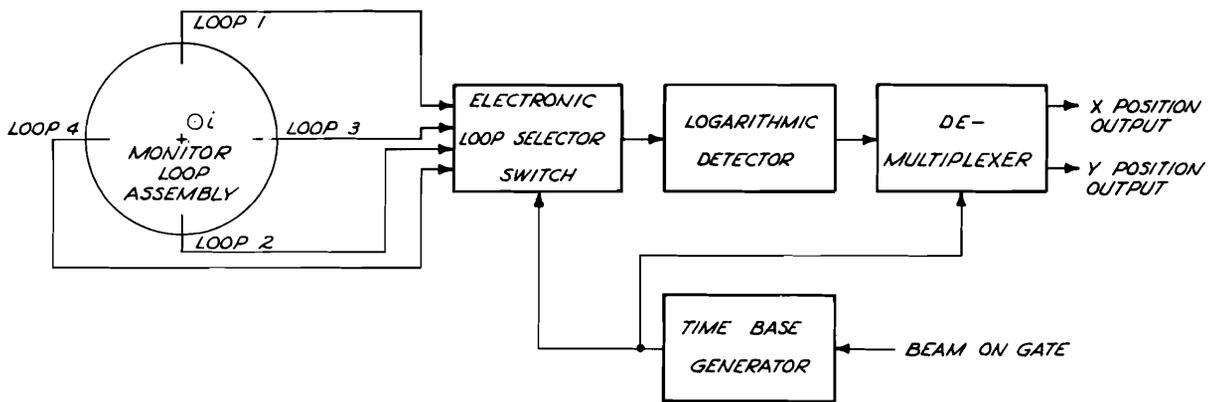
Figure 4. Modified Basic Beam Position Monitor System
