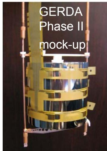
Segmentation of electrodes with individual electronic read-out channels
