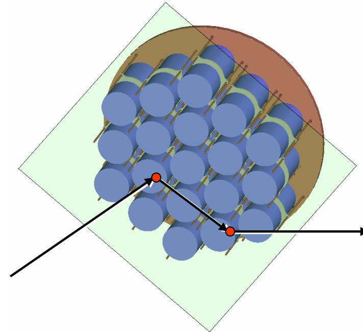
**Granularity cut:** Simultaneous signals in two or more crystals are rejected as  $0\nu\beta\beta$  candidate events
