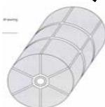
GERDA array with 21 detectors with  $6\phi\text{-}3z$  segmentation
