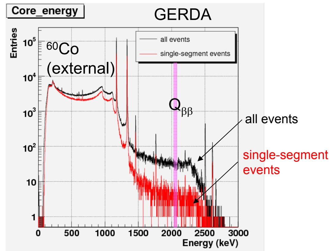
First test data with 18-fold prototype detector in standard cryostat (June)
