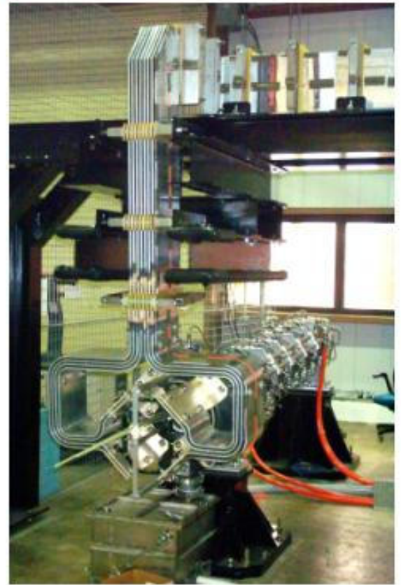
Prototype horn 1 in test stand
