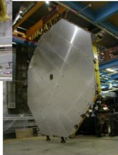
Crane carries plane down the hall for installation
