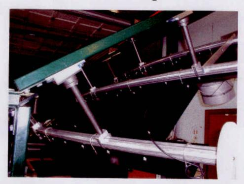
Panels attached to lats carry the PMTs
