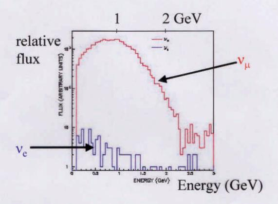
50 m decay length flux in detector located at 500 m
