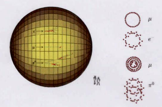
PID based on ring id, track extent, ratio of prompt/late light Signatures substantially different from LSND due to
