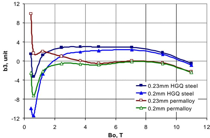
Figure 13. Corrected sextupole field component  $b_3$  vs. the magnet central field for different strip materials and thicknesses in the first excitation cycle.
