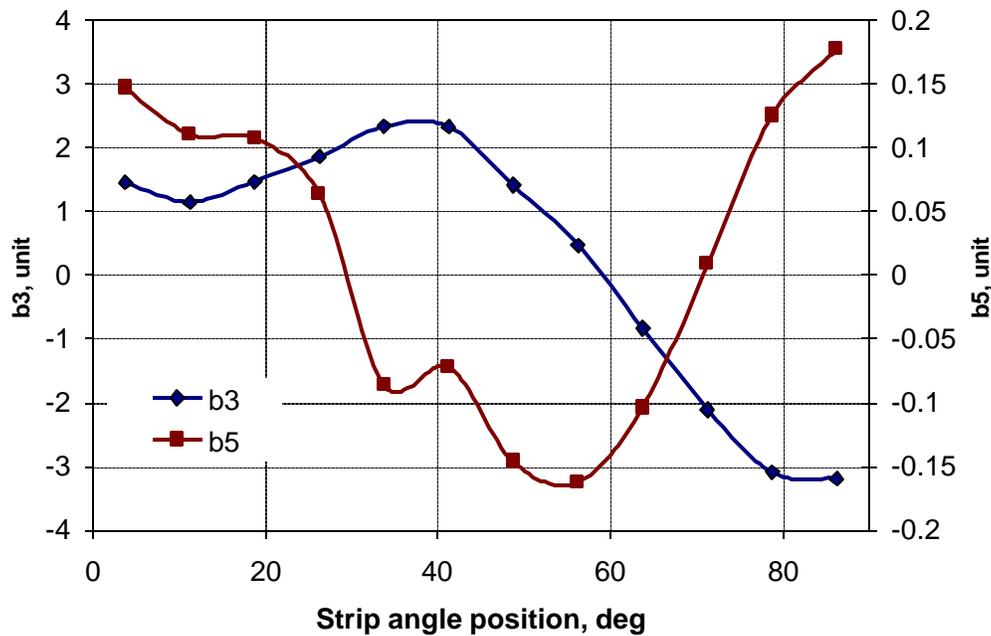
Figure 7:  $b_3$  and  $b_5$  vs. strip azimuthal position for the correction strips installed between the coil and the iron yoke.
