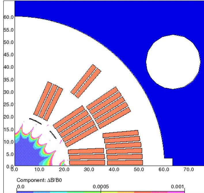
Figure 10: Optimized position of the correction strips and field distribution in the magnet bore.
