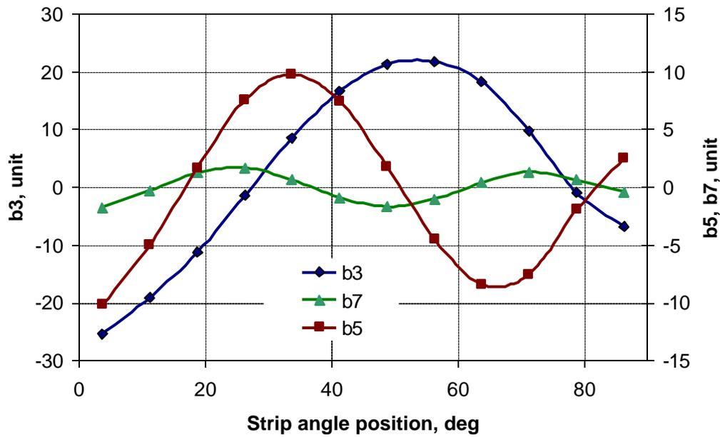
Figure 8: b3, b5 and b7 vs. strip azimuthal position on the beam pipe.
