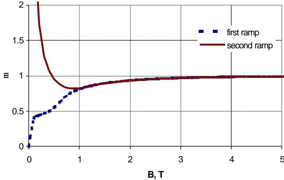
Figure 1: Magnetic permeability of superconducting strand in first and second magnetization cycles.
