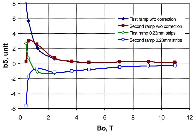
Figure 12: Decapole field component  $b_5$  before and after correction vs. magnet bore field in the first and second cycle.
