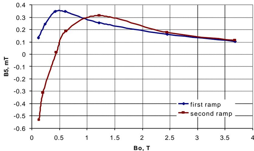
Figure 3: Absolute value of decapole field component vs. magnet bore field in the first and second cycle.
