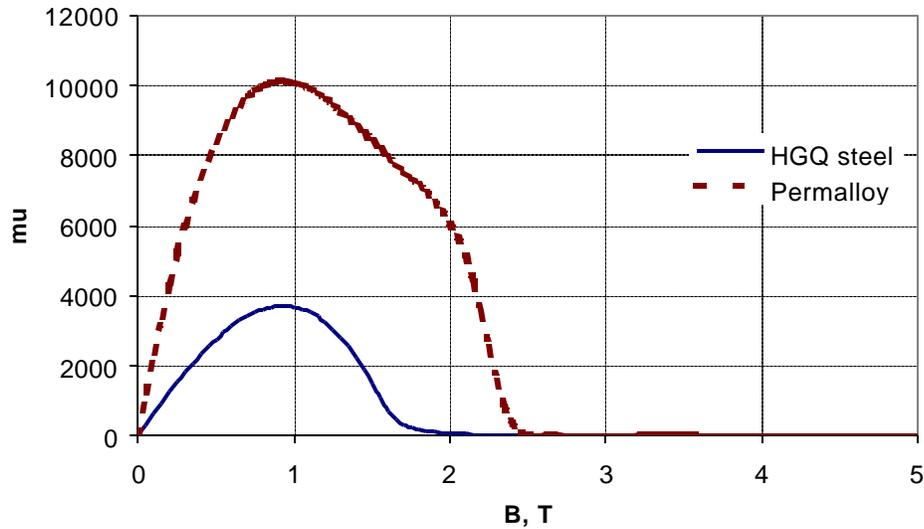
Figure 6: Magnetic permeability  $\mu(B)$  of the strip materials.
