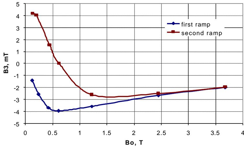
Figure 2: Absolute value of sextupole field component vs. magnet bore field in the first and second cycle.
