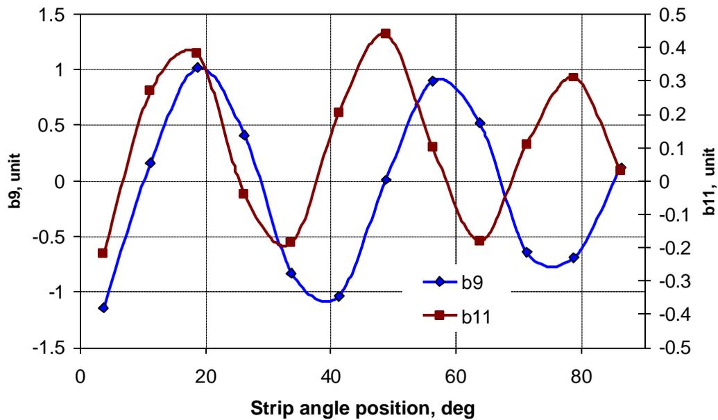
Figure 9: b9 and b11 vs. strip azimuthal position on the beam pipe.
