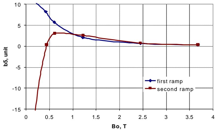
Figure 5: Normalized decapole field component vs. magnet bore field in the first and second cycle.
