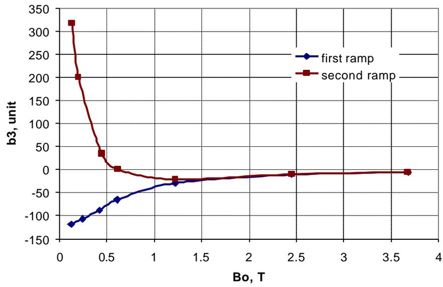
Figure 4: Normalized sextupole field component vs. magnet bore field in the first and second cycle.
