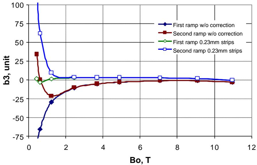
Figure 11: Sextupole field component  $b_3$  before and after correction vs. magnet bore field in the first and second cycle.
