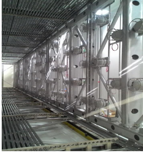
Figure 3.7: Image of the PMT system inside one of the ICARUS TPCs. Taken from Ref. [83].
