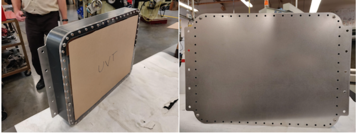
Figure 4.15: The LAPPD watertight housing comprises a 13-inch by 17-inch by 2-inch PVC frame, a UV-transparent acrylic window, and stainless steel backplate. O-rings sit in grooves under the front window and backplate to provide the watertightness needed for the LAPPD system. The backplate offers some level of heat dissipation.
