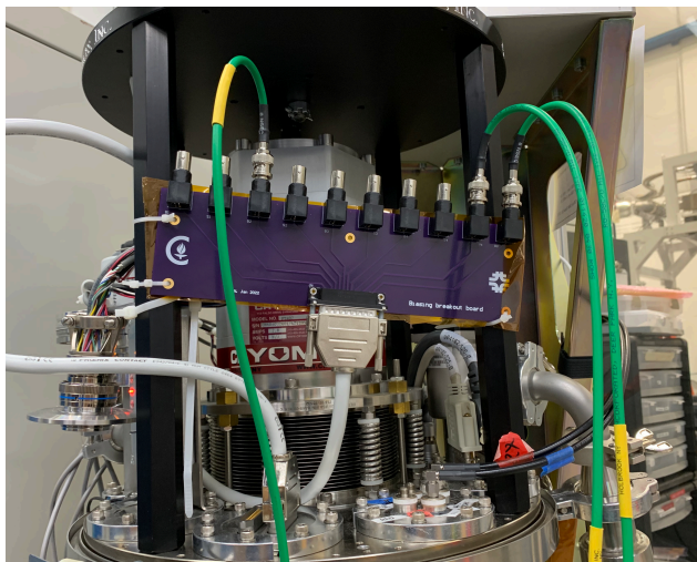
Figure 9.14: The room-temperature biasing breakout board is shown.
