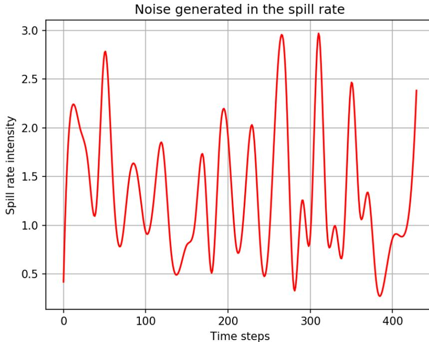
Figure 4.9: Variations in spill intensity generated by the physics simulator using log-normal distribution. We normalize the expectation value of the variations to 1.
