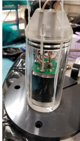
**Figure 5.33:** Left: Schematic cross-section view of the AmBe source. Detection of scintillation light emitted by the gamma in the BGO with the SiPMs provides the tag for the neutron emission. Figure based on [225]. Right: Picture of the AmBe source in the housing.
