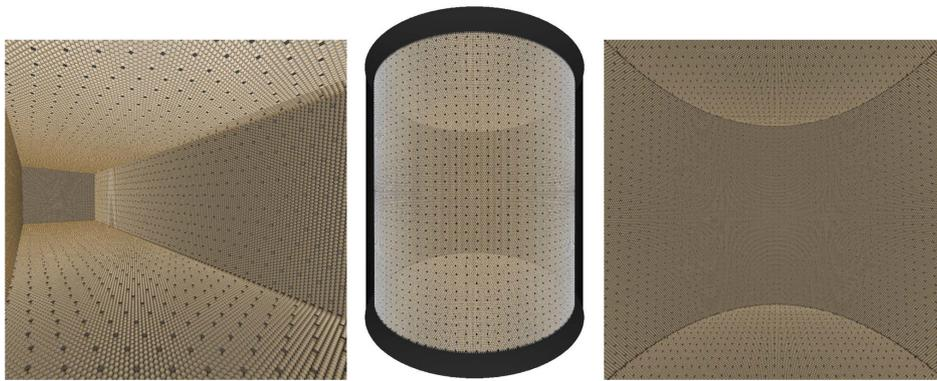
**Figure 8.26:** Schematic depictions of the suggested THEIA detector geometry options. The location of THEIA-25 in one of the DUNE caverns is shown in the top row while the bottom row shows the modeled geometries of THEIA-25 (*left*) and THEIA-100 (*center, right*). Figures taken from [296].
