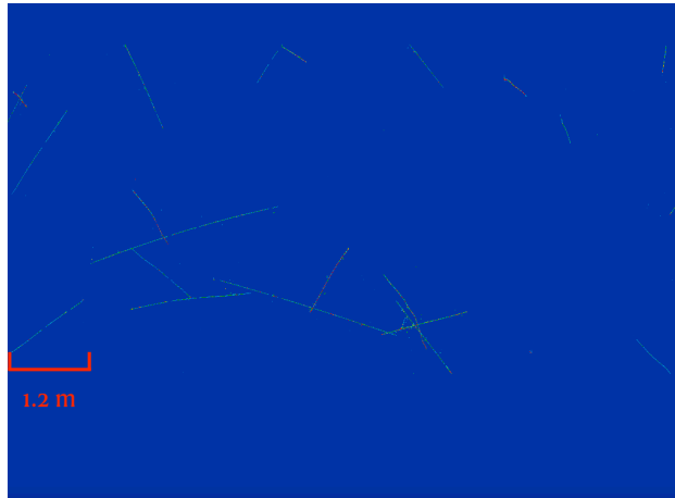
Figure 5.1: An event display with cosmic rays from the MicroBooNE collection plane. Cosmic rays, as shown in this image, are randomly distributed in position in the detector (the x -axis represents the detector z -axis direction) and time (the y -axis) in an event.
