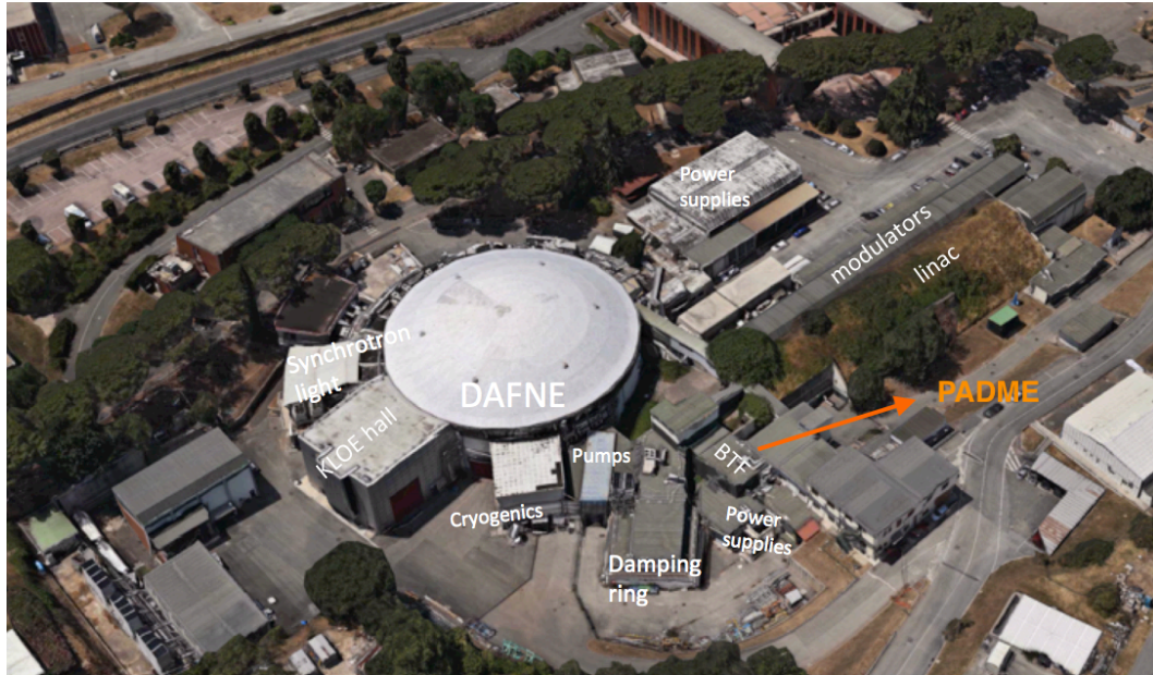
Figure 13.4: Bird's-eye view of the DAFNE complex and the location of the PADME experiment at the BTF (test beam line) [116].
