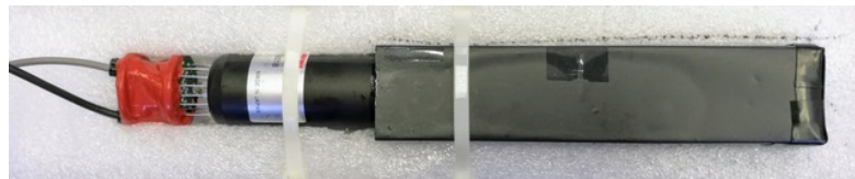
Figure 14.9: Photo of the PMT and crystal setup for the SAC test beam. A \text{PbF}_2 crystal is coupled to the R13478UV PMT via optical grease.
