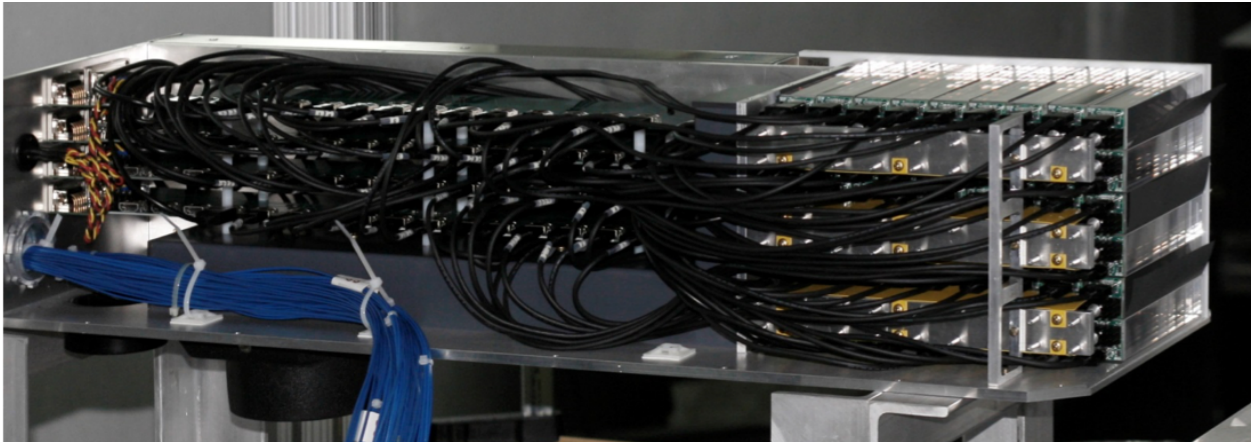
Figure 4.27: The inside of the production calorimeter tested at SLAC in June 2016. There are 54 \text{PbF}_2 crystals, each black-wrapped, in a 6 \times 9 array. The crystals are all to the right side of the photo; most of the space inside the calorimeter housing is dedicated to electronics.
