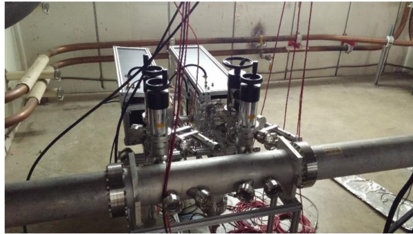
Figure 1.13: A picture of the SEY test stand in the Fermilab Main Injector
