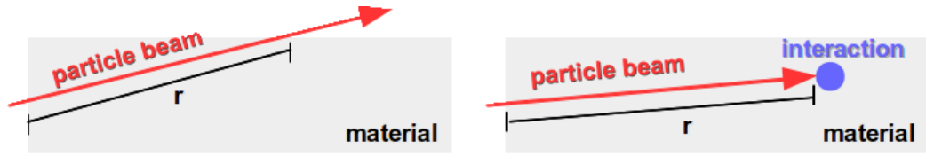
FIG. 4.1: Particle beam traversing a volume. Left side: particle leaving the volume without interacting. Right side: particle interacting in the volume.
