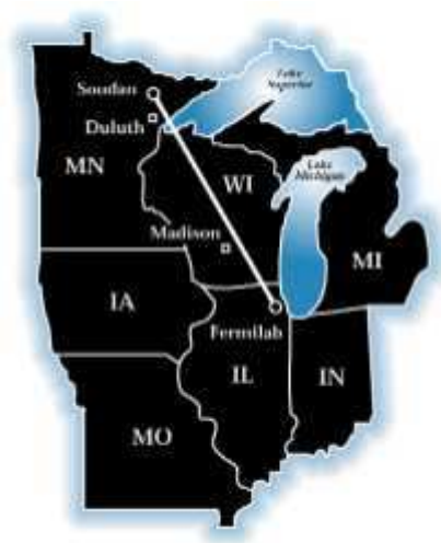
Figure 3.1: A geographical picture of the MINOS experiment. Neutrinos are produced at Fermilab and go through the Near detector, measuring the unoscillated energy spectrum, then the neutrinos travel 735 km to Soudan mine to be detected, in their oscillated form, at the Far detector.
