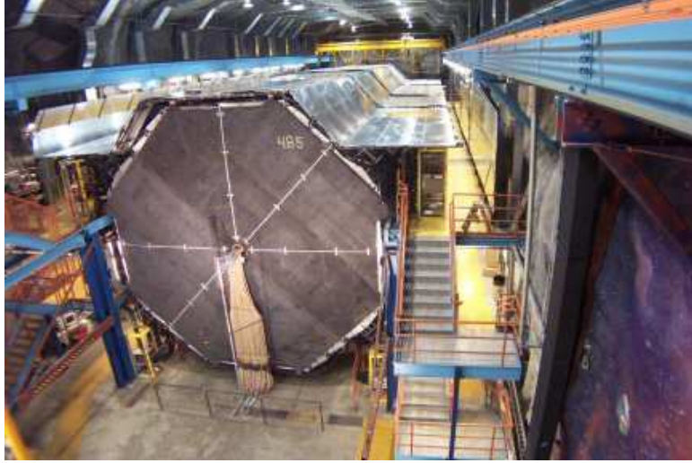
Figure 3.9: A picture of the Far Detector at Soudan Mine, Minnesota.
