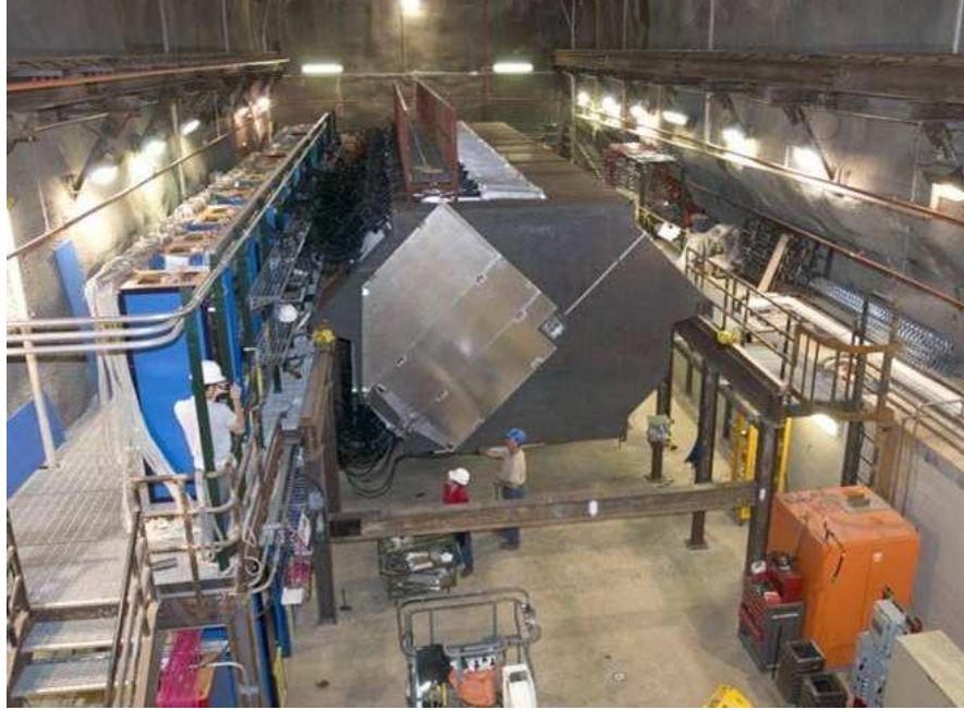
Figure 3.8: The Near Detector during plane installation. The exposed first detector plane is partially instrumented with scintillator modules. The beam centre is located to the left of the coil hole, in the centre of the visible scintillator modules. Electronics racks are visible on the left of the detector.
