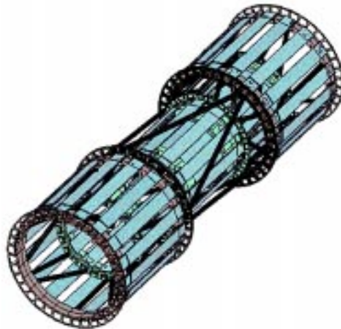
Figure 1.6: Overall ISL assembly. The readout modules are installed on a carbon fiber structure also containing the SVXII detector.
