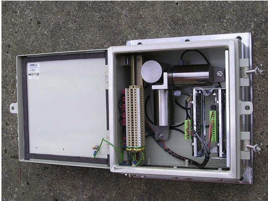
Figure 6.10: Sensonics model SA-3 safety seismic switch
