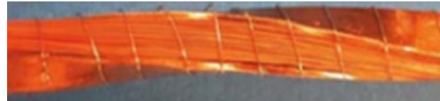
Figure 1: A view of a Twisted Stacked Tape cable [5].
