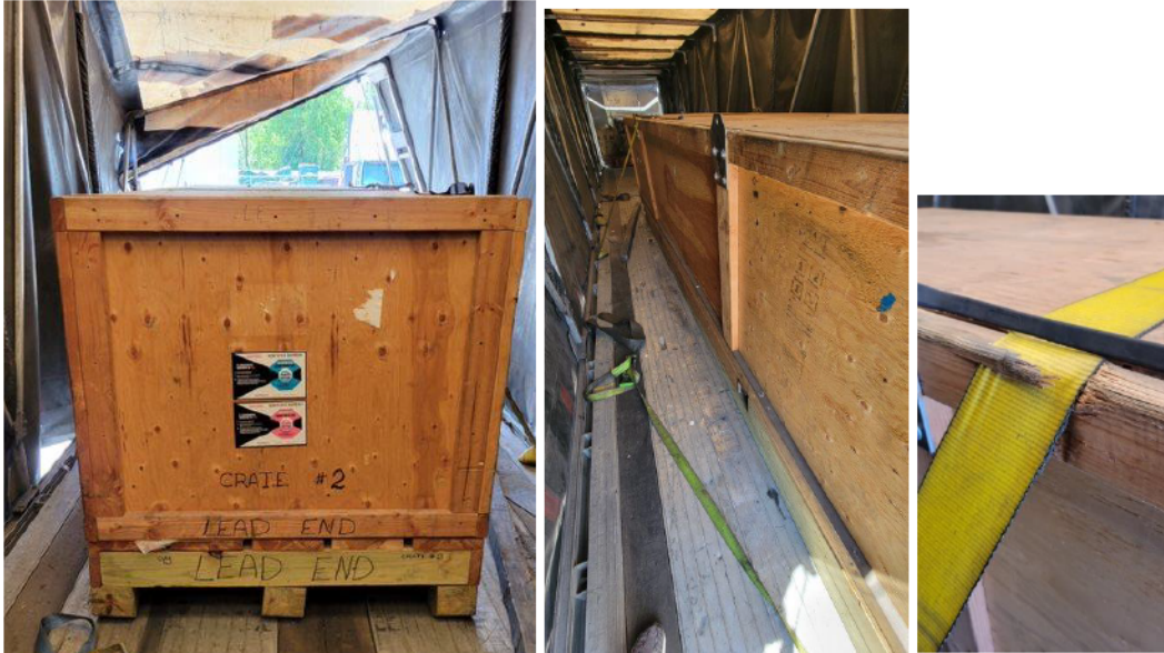
Figure 1: Left to right: Photo of the lead end of the crate/magnet taken after the incident from the cab end of the trailer; The yellow sling was found close to the metallic tab; detail of the yellow ling after the incident
