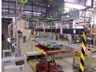
Figure 12: Photo of T-1043 setup showing CRV dicounters mounted on the movable table.
