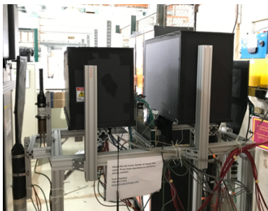
Figure 50: Photograph of the setup with two dark-boxes housing two Incom LAPPDs, positioned outside of the enclosure behind the pion beam dump.
