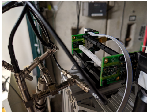
Figure 24: Example of test-beam setup for telfon-wrapped LYSO bars with dual SiPM readout.
