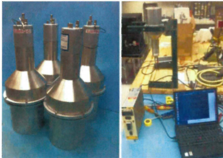
Figure A.2: EJ-301 neutron detector array (left) and its DAQ (right). We demonstrated the performance of the EJ-301 detector for neutron flux measurement at BNB in reference [29].
