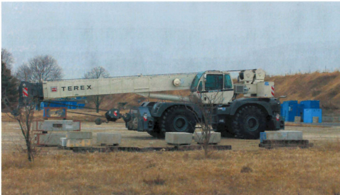
Figure A.4: Heavy duty (70 ton lifting power) crane at Fermilab. The crane will be available for the proposed concrete shielding work.
