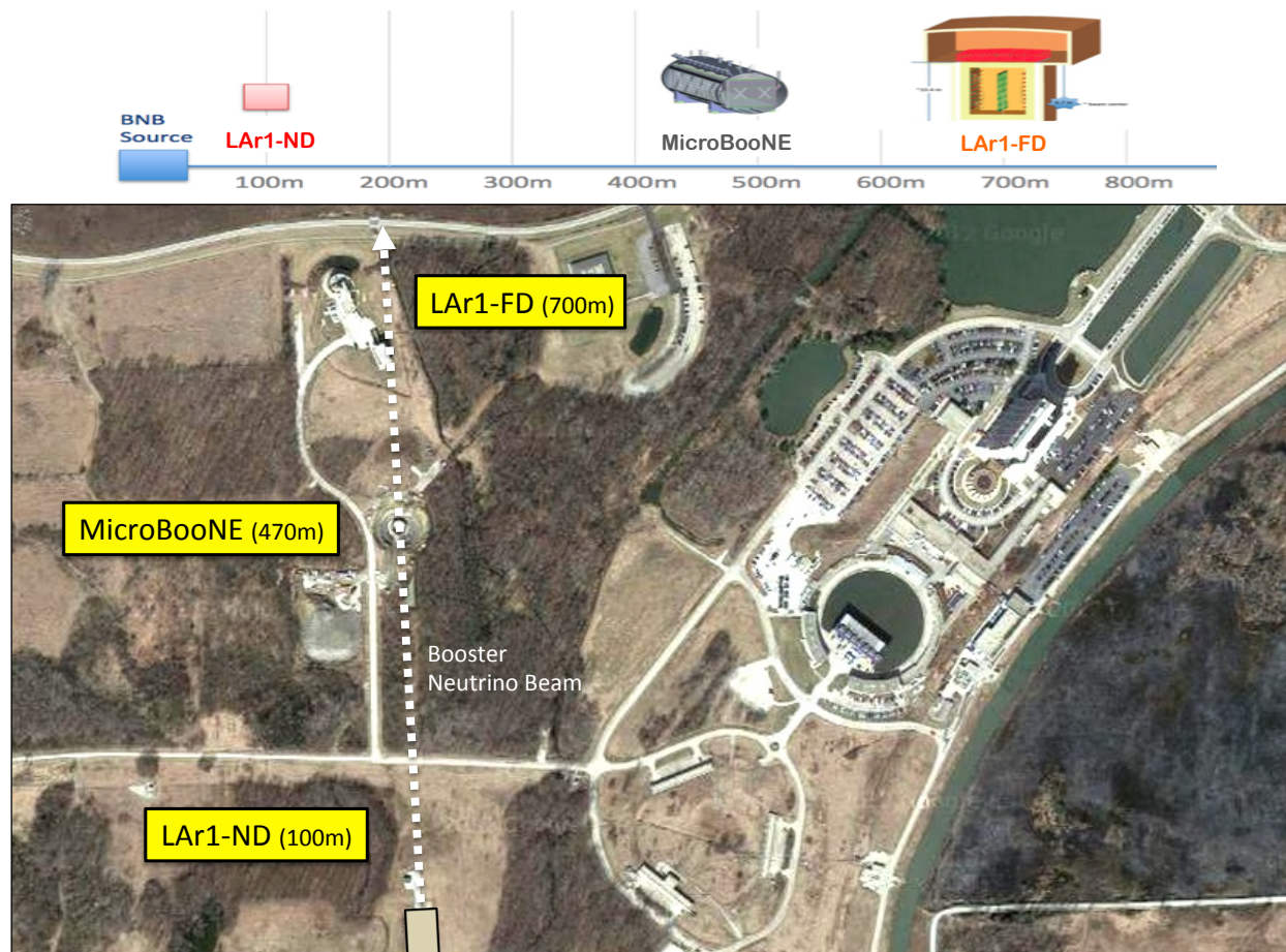
Figure 1.2: Aerial view of the Fermilab Booster Neutrino Beam showing the locations of the MicroBooNE detector (currently under construction), the proposed LAr1-ND, and a possible future kiloton-scale LAr TPC detector, LAr1-FD.
