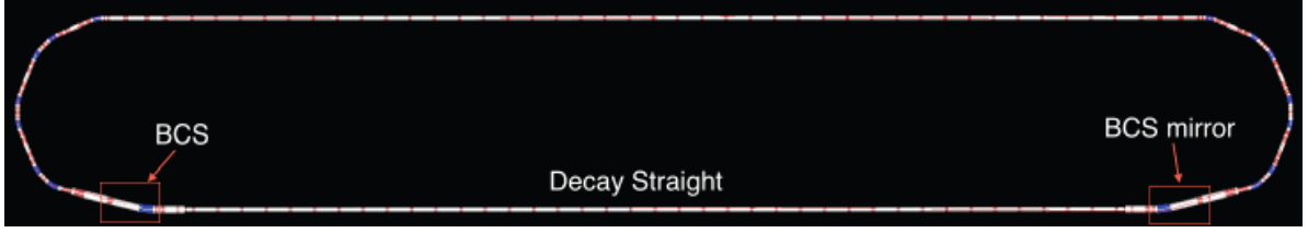
Figure 44. Racetrack ring layout. Pions are injected into the ring at the Beam Combination Section (BCS). Similarly, extraction of pions and muons at the end of the production straight is done using a mirror image of the BCS.
