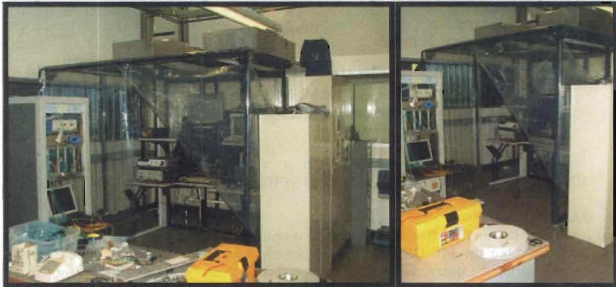
Fig. 3. Example of the unistrut clean tent that the experimenters would like to build in the Minos hall. The picture was taken from a similar tent located at SiDet.
