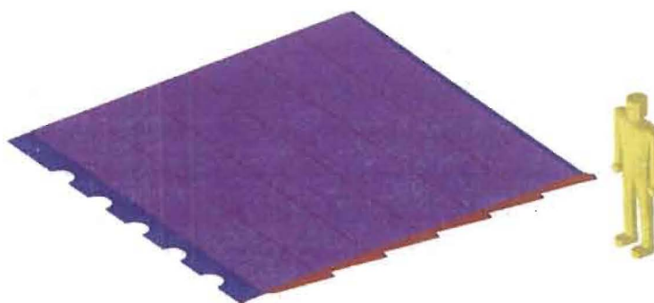
Figure 4.11: A completed x layer with six cans of scintillator and a 0.50 inch thick steel backing. The assembly weighs 2.2 tons. Cans are attached to the steel backing by bolts at the ends of the can, and a strap (not shown) similar to the MINOS design which prevents the cans from bending away from the backing in the middle.
