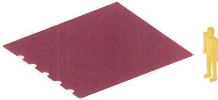
Figure 4.21: A typical filler module for section 4. Not shown on any of the module pictures are lifting lugs to place the modules in the stack. The ears that allow the plates to hang from the support structure are welded on tabs.
