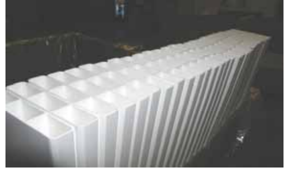
Fig. 6.6: Cell structure of the three cell prototype of extruded PVC with 12% TiO_2 .
