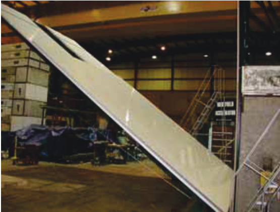
Fig. 15.1: The “half-size” prototype of NOvA at Argonne National Laboratory. The prototype is ~ 8 meters high and it is made of two layers of extrusions. The planes were assembled on a Unistrut strongback and winched up against the vertical bookend on the right while pivoting about the lower right corner.
