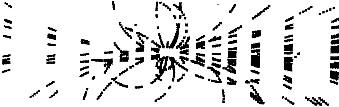
Figure 51: A typical TEV I event from the b\bar{b} two-jet process, showing all minivectors in the straw tracking system.
