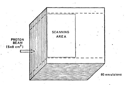
Fig. 1 Layout of the proposed stack of 80 pellicles of Ilford G5 emulsions exposed to a beam of 300 GeV protons having a uniform illumination over  $5 \times 8 \text{ cm}^2$ .
