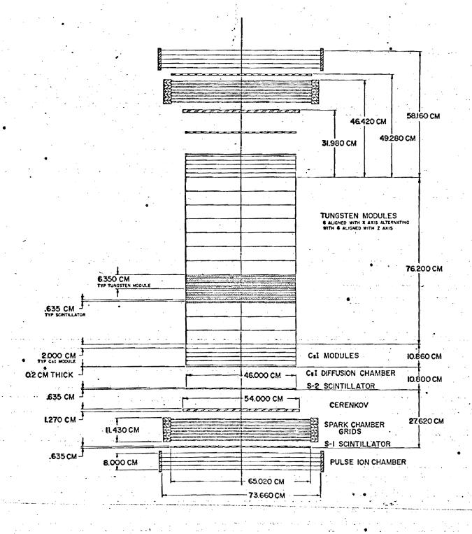
Figure 1. Schematic diagram of experiment showing dimensions.
