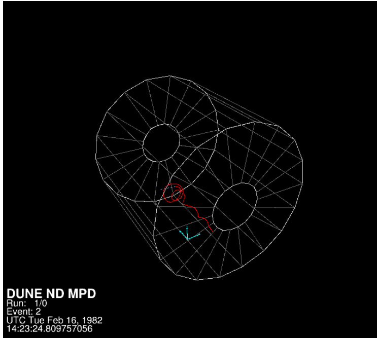
FIG. 11. A 30 MeV \nu_e CC interaction in a 5-bar gaseous Ar TPC in a 0.1T magnetic field. The final-state electron shown in the figure has an energy of 15 MeV.
