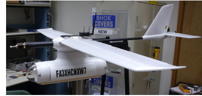
Figure 3: Beam calibration drone in development at Brookhaven National Laboratory.
