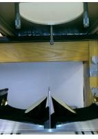
Figure 44: Reflectometer setup at University of Michigan. The reflectometer uses a variable microwave source to measure the reflection off a flat sample. An off-axis parabolic mirror collimates the beam from the source and directs the beam at the sample. Another mirror collects the beam and directs it at a horn-coupled photodiode. Calibrating with known highly reflective sources, this set-up can measure absolute reflection down to 0.1%, with a relative accuracy of a few percent.
