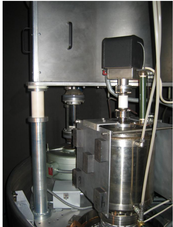
Figure 8. Mechanical schematic and photo of the beam collector installed in the Pelletron terminal. In the drawing: 1- Suppressor electrode, 2- water-cooled collector surface, 3- ion pump, 4- HV insulator, 5- terminal platform, 6 – collector solenoid. The steel plates and magnets creating the transverse magnetic field in the collector are not shown. Visible in the photo: the collector with steel plates and magnets (right); the generator (behind the collector) installed on the axis of the rotating shaft; a platform at the cathode potential (covered, top); an insulated part of the shaft (translucent cylinder above the generator) connected to another generator supplying power to electronics at the platform. The terminal shell is lifted.
